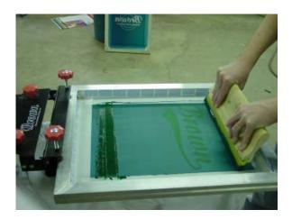
D. Place the squeegee blade at the rear of the image with the front edge of the blade at a slight forward angle to screen. The handle of the squeegee should be pointing at you with the blade pointing toward the back of the screen.
