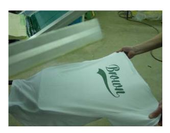
The flash unit should be set on "high" and be approximately 3" away from the garment. It will take anywhere from 5 to 20 seconds to flash an ink. Remember that you are not trying to cure the ink on the shirt. Over flashing will cause its own list of problems
