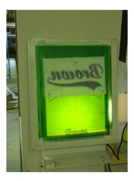
B. Place the frame onto your viewing table over your MAP. By using transparent tape, attach your first color separation to your screen taking care to match the registration marks to each other.
